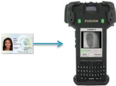
Authentication at the scene of a disaster requires the first responder to present their card to a FIPS-201-compliant handheld reader. The reader allows for the check of the PIN, facial image stored on the chip and the fingerprint stored on the chip.
