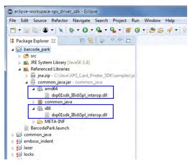
Verify that dxp01sdk\_IBidiSpl\_interop.dll displays for both 32-bit and 64-bit systems.
