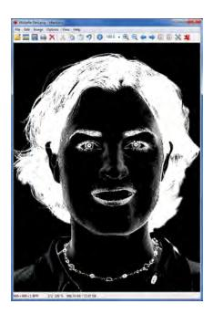
5. Select **Replace Color** from the **Image** menu. Replace the source color (black) with the new color (RGB:217,217,217) in the Replace Color dialog box. The Card Printer Driver recognizes 217:217:217 as the UV "color" and prints those elements using the UV panel of the ribbon.
