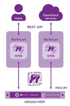
Entrust nShield Connect hardware security module (HSM) protects the storage, transport, and secure keys used by the Red Hat Barbican OpenStack common KMS. nShield HSMs can be deployed on-premises or as a service.
