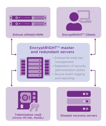
nShield Connect HSMs integrate with Prime Factors EncryptRIGHT to safeguard and manage underpinning master keys used to protect data. nShield can be deployed on-premises or as a service.
