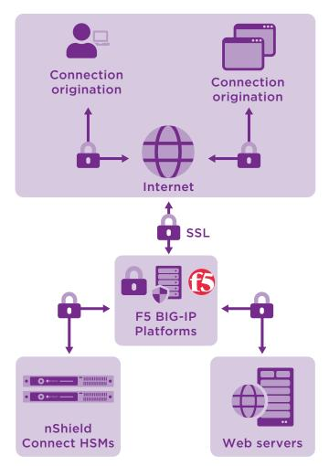
Entrust nShield® Connect hardware security modules (HSMs) integrate with F5 BIG-IP application delivery controllers (ADCs) to protect SSL encryption/decryption keys and certificates. nShield HSMs can be deployed on-premises or as a service.
