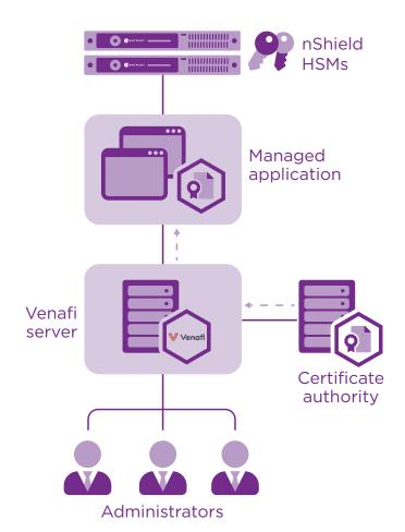
The Venafi Trust Protection Platform delivers key and certificate orchestration with the key pairs securely maintained by the Entrust nShield HSMs, deployed on-premises or as a service.
