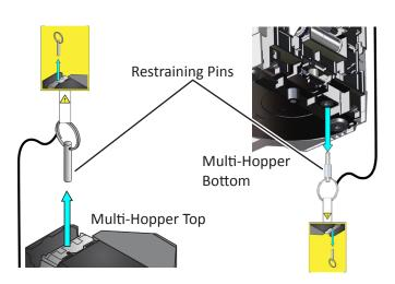
Save the restraining pins after removing them from the multihopper. They are required if you need to repackage and return the multi-hopper for service.
