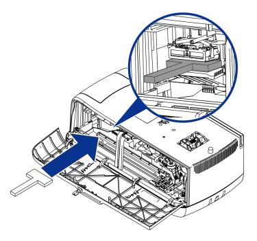
b. Push the transport assembly towards the back of the embosser and insert the hard foam block to secure the assembly.
