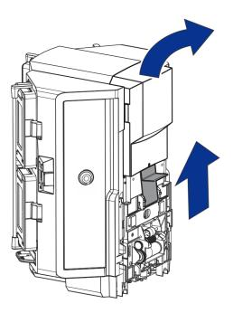
b. Insert the restraining pins at the top and bottom of the mutli-hopper to secure the elevator inside the multi-hopper for shipping.
