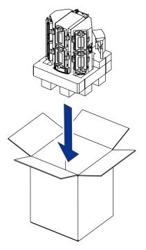
C. Place the top foam cap in the shipping carton on top of the multi-hopper.
