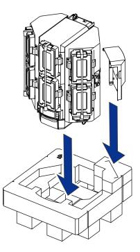
b. Lift the multi-hopper with the bottom foam cap into the shipping carton.
