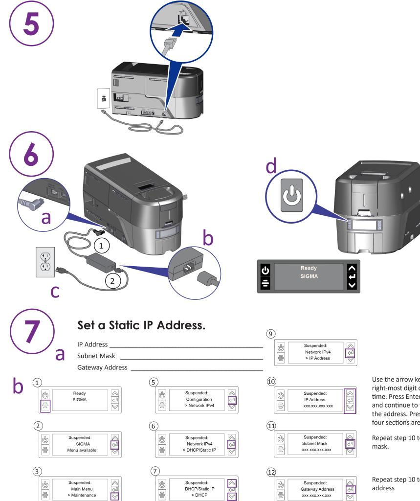
Use the arrow keys to change the right-most digit one number at a time. Press Enter to save each value and continue to the next section of the address. Press Enter when all four sections are correct.
