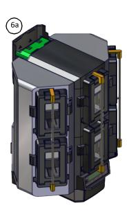
b. Insert the restraining pins saved from the printer's installation at the top and bottom positions of the multi-hopper to secure the elevator and shuttle.
