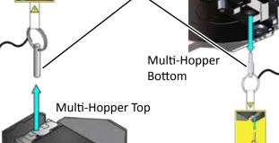
Save the restraining pins after removing them from the multihopper. They are required if you need to repackage and return the multi-hopper for service.
