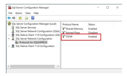
5. Open the firewall port 1433 for the TCP/IP connection to the MS SQL server.
