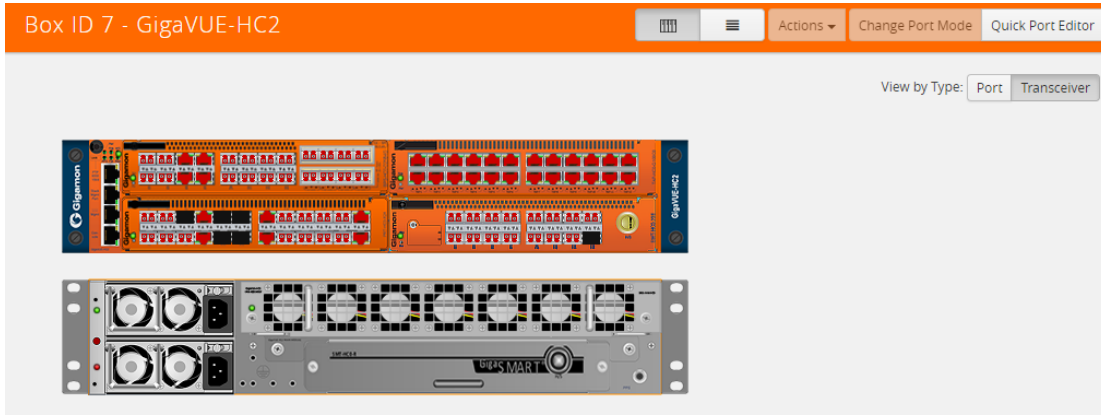
Figure 119 Chassis view of GigaVUE-HC2 with TAP-HC0-G100C0 Module
