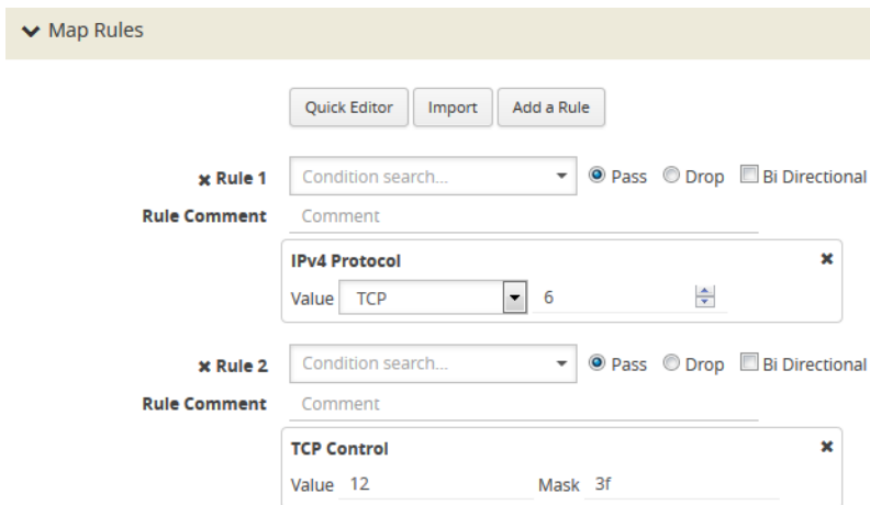
Figure 37 Map Rule Matching All Packets with Both ACK and SYN Bits set
