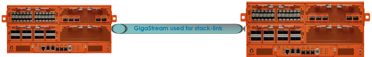
Figure 4 Daisy-Chain Configuration using GigaStream for Stack-link
