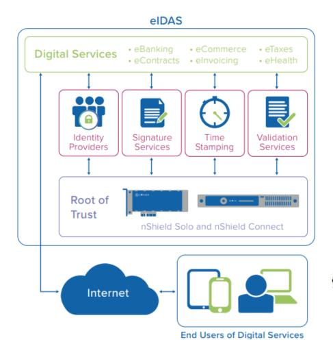
nShield hardware security modules (HSMs) let you generate and manage your encryption and signing keys while protecting them in certified, tamperresistant hardware.
