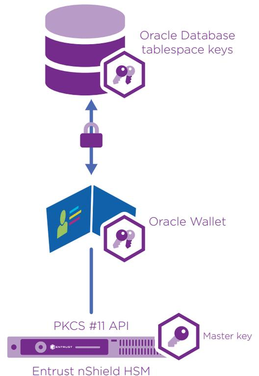
Entrust nShield hardware security modules (HSMs) safeguard and manage the master encryption key (MEK) used by Oracle Database Wallet.
