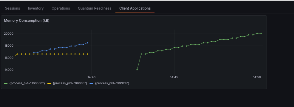
Figure 10: Dashboard - Client Applications (memory leak detection)
