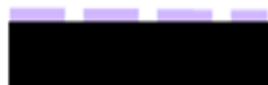
UV dashed line printed behind a black rectangle—the black prints over the UV element
