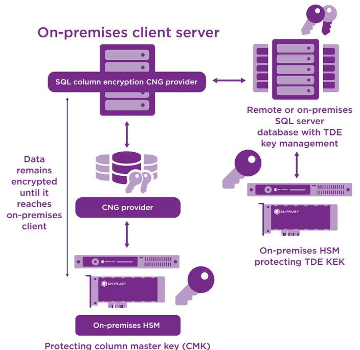
Entrust nShield hardware security modules (HSMs) protect and manage the column master key (CMK) that wraps the column encryption keys (CEKs) that encrypt the data.
