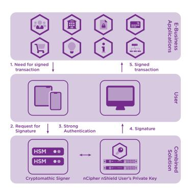
Entrust nShield\* Connect HSMs safeguard and manage the private key used by Cryptomathic Signer to deliver Qualified Electronic Signatures to online banking customers. nShield HSMs can be deployed on-premises or as a service.
