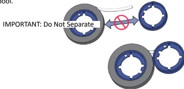
4. Match the supply spool hub with the left side spindle.
