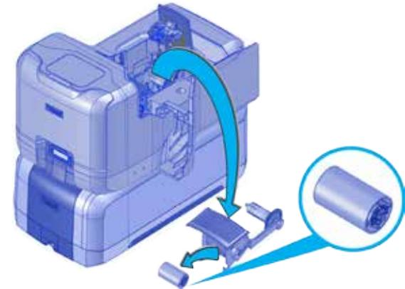
5. Slide the spindle into the cleaning sleeve (a).
