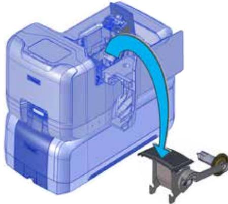
4. Load a full roll of print ribbon (blue spool) onto the spindle closest to the cartridge handle until it clicks into place.
