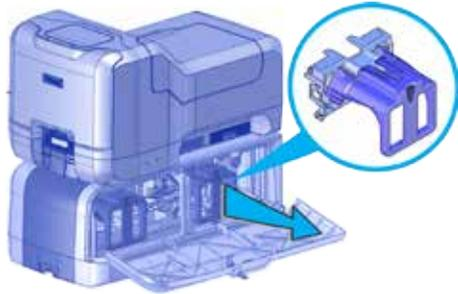
3. Remove the new indent roll from its package.
