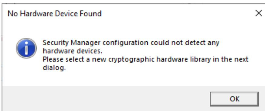
Click the **OK** button. A new dialog opens where you can select the driver file to be used to connect to the HSM – choose `mpcm-pkcs11.dll` from the directory where the Trident HSM files are located (in our example `C:\trident`). If the Entrust Configuration Tool successfully recognized the driver library, in the next step you have to select the slot you want to use.
