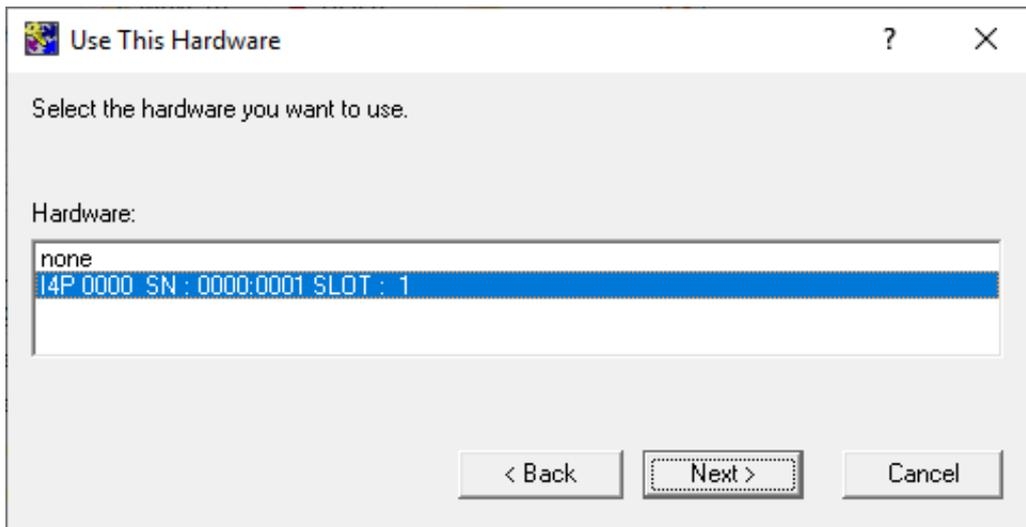
Select the row representing the appropriate slot and click **Next**. In the following steps you have to specify the various characteristics of the Certificate Authority key and its management; see the Entrust Security Manager installation guide for the meaning and effect of these parameters. It is important to ensure that you set a key type which is compatible with Trident HSM.
