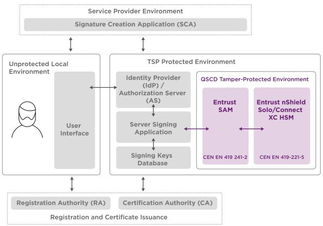
Example of server signing system implementation with a QSCD including the Entrust SAM and the Entrust nShield Solo XC or Connect XC HSM. The architecture shows a simplified workflow focusing on the QSCD.
